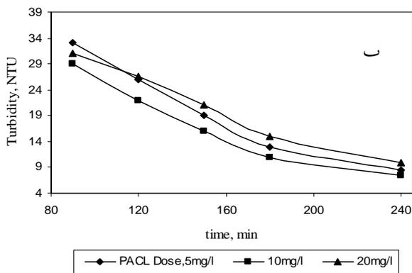
**PACL effectiveness on effluent turbidity in different detention times (inlet turbidity=20 NTU)**
